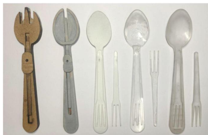
Fig.7: Materials exploration such as MDF, acrylic sheets, and HIPS sheets
